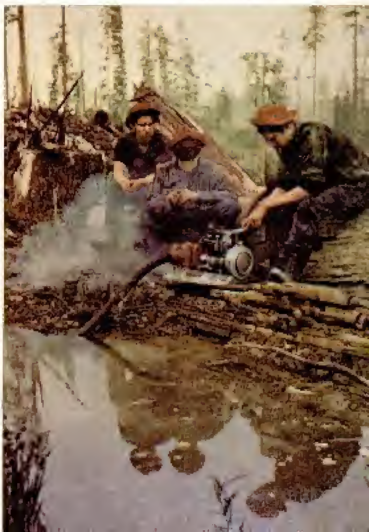
Tree-farm workers take a breather beside portable fire pump which sucks water from pond in Northwest
